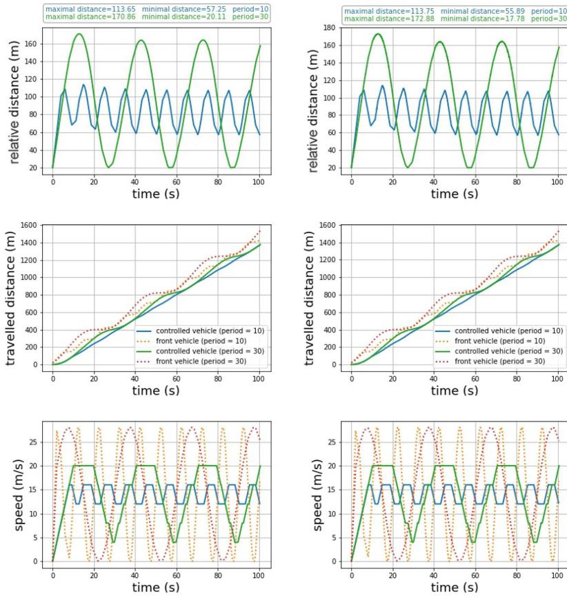
**Fig. 11.** Simulation results for the synchronous (left part) and the asynchronous controller (right part) for  $T_f \in \{10\text{ s}, 30\text{ s}\}$  and  $n = 8$  speed levels and sensing period  $T = 0.02\text{ s}$ .
