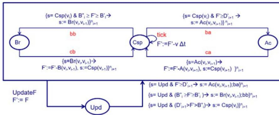
Fig. 9. Extended automaton modelling the asynchronous controller
