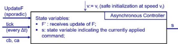
Fig. 8. Inputs and outputs of the asynchronous controller
