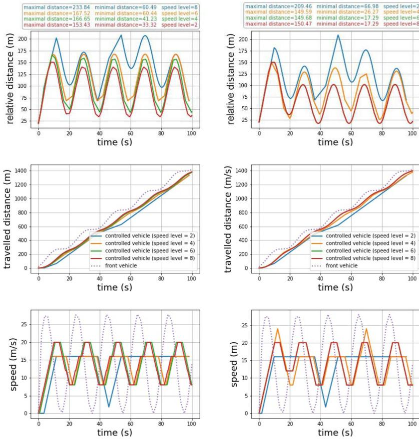
**Fig. 15.** Simulation results for the synchronous controller with and without considering the braking distance of the front vehicle (right and left part, respectively) for four different speed levels  $n \in \{2, 4, 6, 8\}$ .
