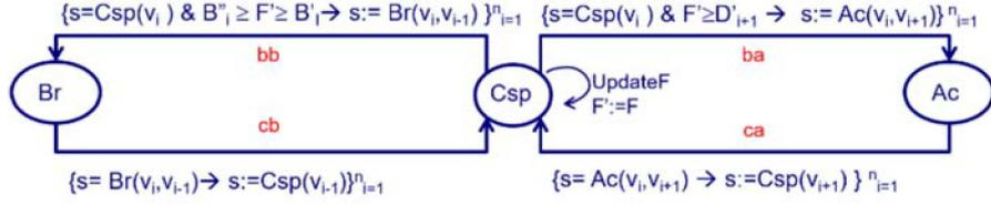
Fig. 6. Extended automaton modelling the synchronous controller
