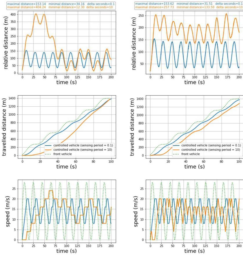
**Fig. 13.** Simulation results for the synchronous (left part) and the asynchronous (right part) controller for two different sensing periods ( $T \in \{0.1 \text{ s}, 10 \text{ s}\}$ ) and  $T_f = 20 \text{ s}$ ,  $n = 8$ .
