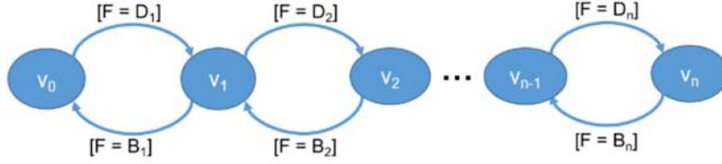
**Fig. 5.** Automaton modelling the collision avoidance principle
