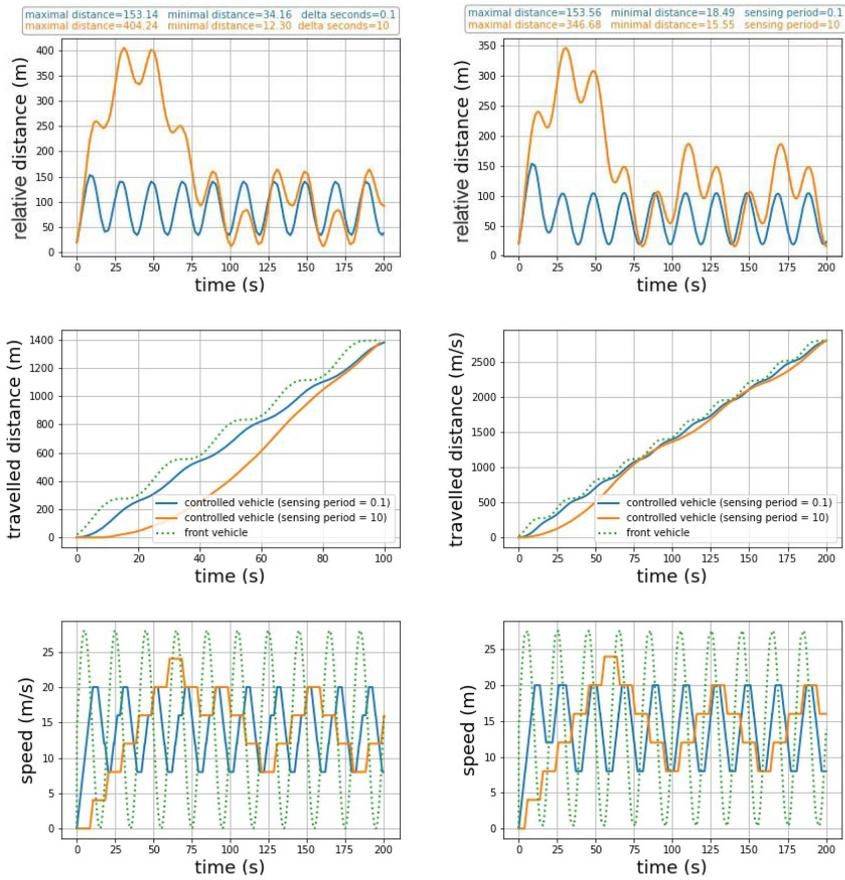
**Fig. 16.** Simulation results for the synchronous controller with and without considering the braking distance of the front vehicle (right and left part, respectively) for two sensing periods  $T \in \{0.1 \text{ s}, 10 \text{ s}\}$ .
