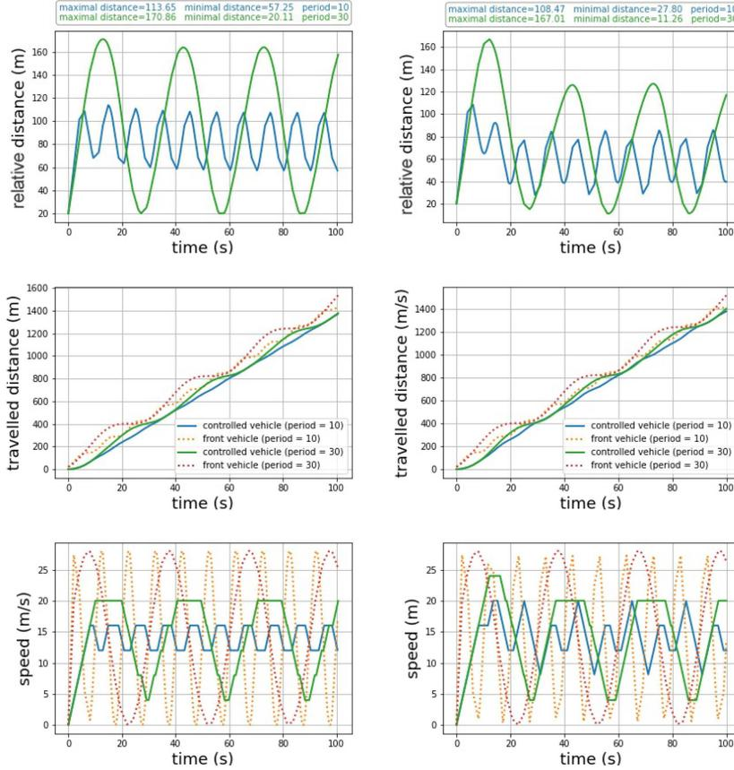
**Fig. 14.** Simulation results for the synchronous controller with and without considering the braking distance of the front vehicle (right and left part, respectively) for  $T_f \in \{10 \text{ s}, 30 \text{ s}\}$ .
