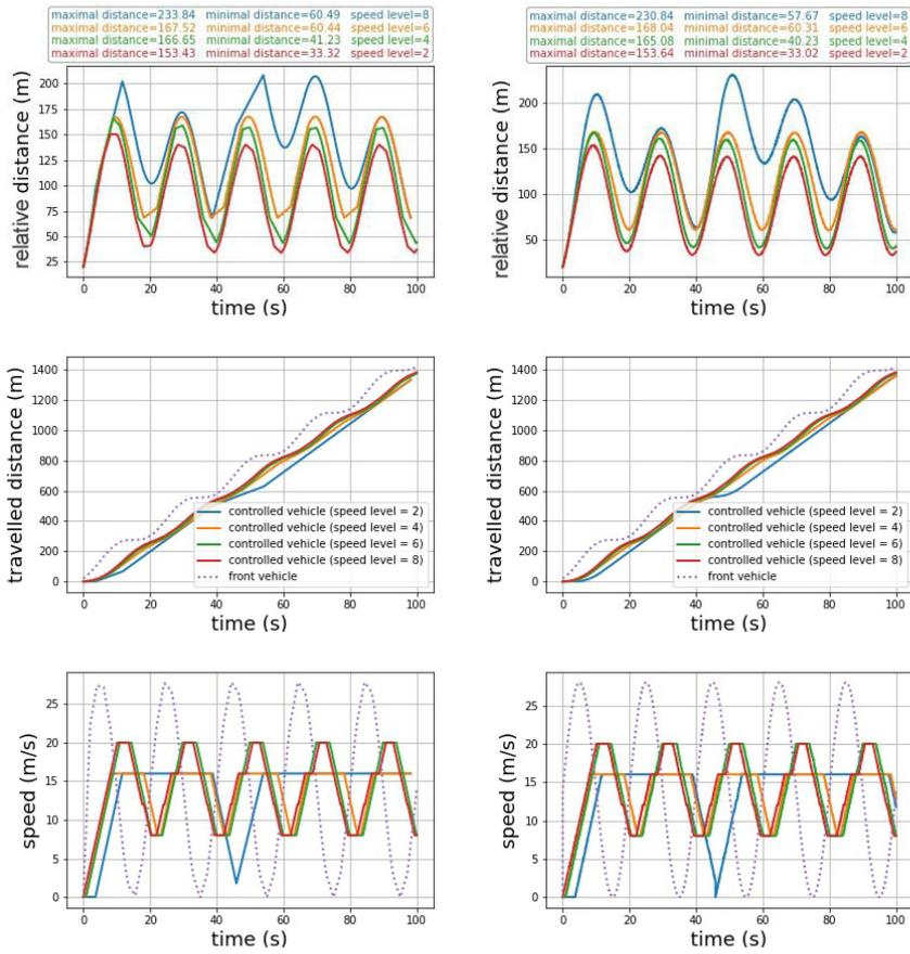
**Fig. 12.** Simulation results for the synchronous (left part) and the asynchronous (right part) controller for four different speed levels ( $n \in \{2, 4, 6, 8\}$ ) and  $T_f = 20$  s,  $T = 0.02$  s.
